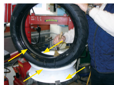
Fig. 1: Lubricating the tire and rim.
