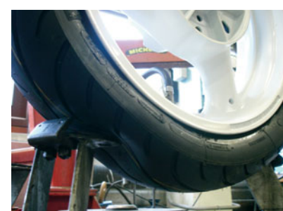
Fig. 6: Apply pressure to establish a seal if needed.
