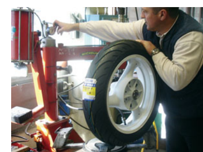
Fig. 3: Installing the second bead.
