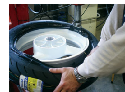
Fig. 4: Applying pressure to avoid stretching.
