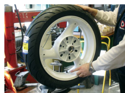
Fig. 5: Position uninflated tire vertically.
