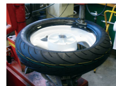
Fig. 3: Installing the second bead.
