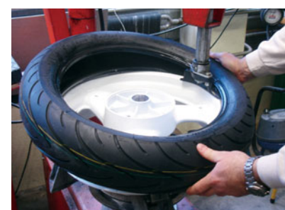
Fig. 2: Installing the first bead.
