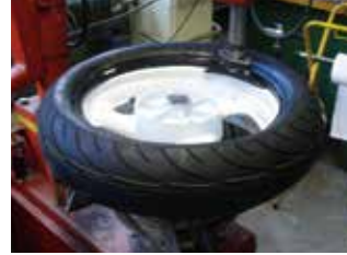
Fig. 3: Installing the second bead.
