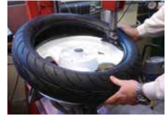
Fig. 2: Installing the first bead.
